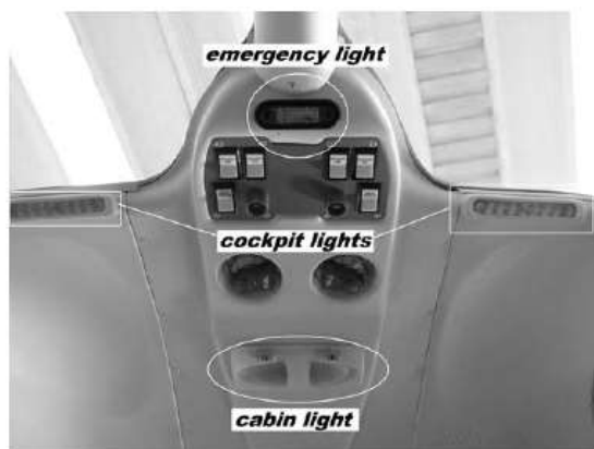
Figure 9. – Over-head panel lights arrangement
